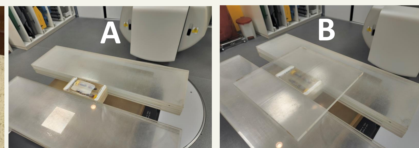
Figure 2. Irradiation setup under LINAC: mini-phantom surrounded by PMMA plates (A) and covered with a PMMA plate (B)
