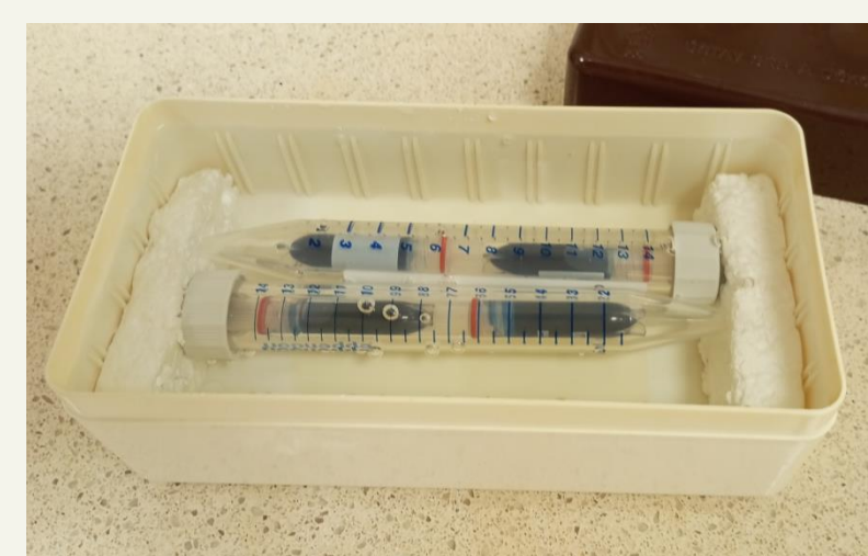
Figure 1. Blood samples in secondary containers, placed into the mini-phantom, all filled with water
