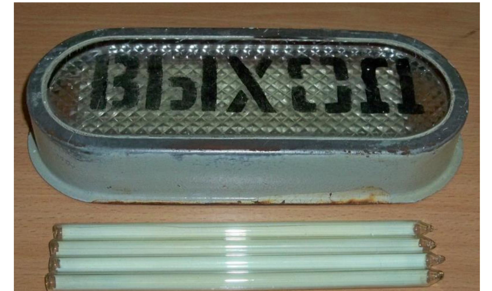
Fig. 1 The tritium self-luminous sign. Next to the sign are placed fluorescent elements (glass tubes with gaseous tritium)
