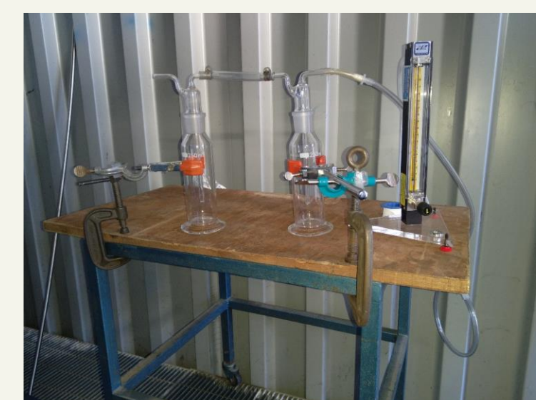
Figure 4-a. Set of instruments to spill the gaseous CO 2 by the SKID
