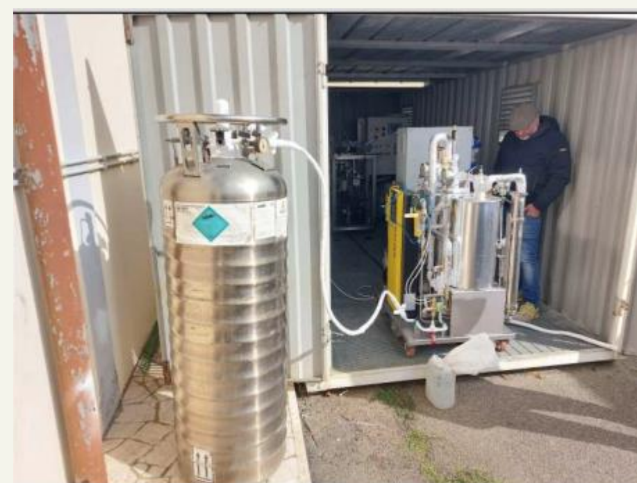
Figure 1. The SKID with the 180 L dewar of liquid nitrogen
