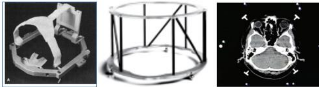
Figure1. Stereotactic GTC frame b) BRW localizer CT frame; axial patient image with 9 rods visible CT localizer and axial CT image of a patient (BPU)
